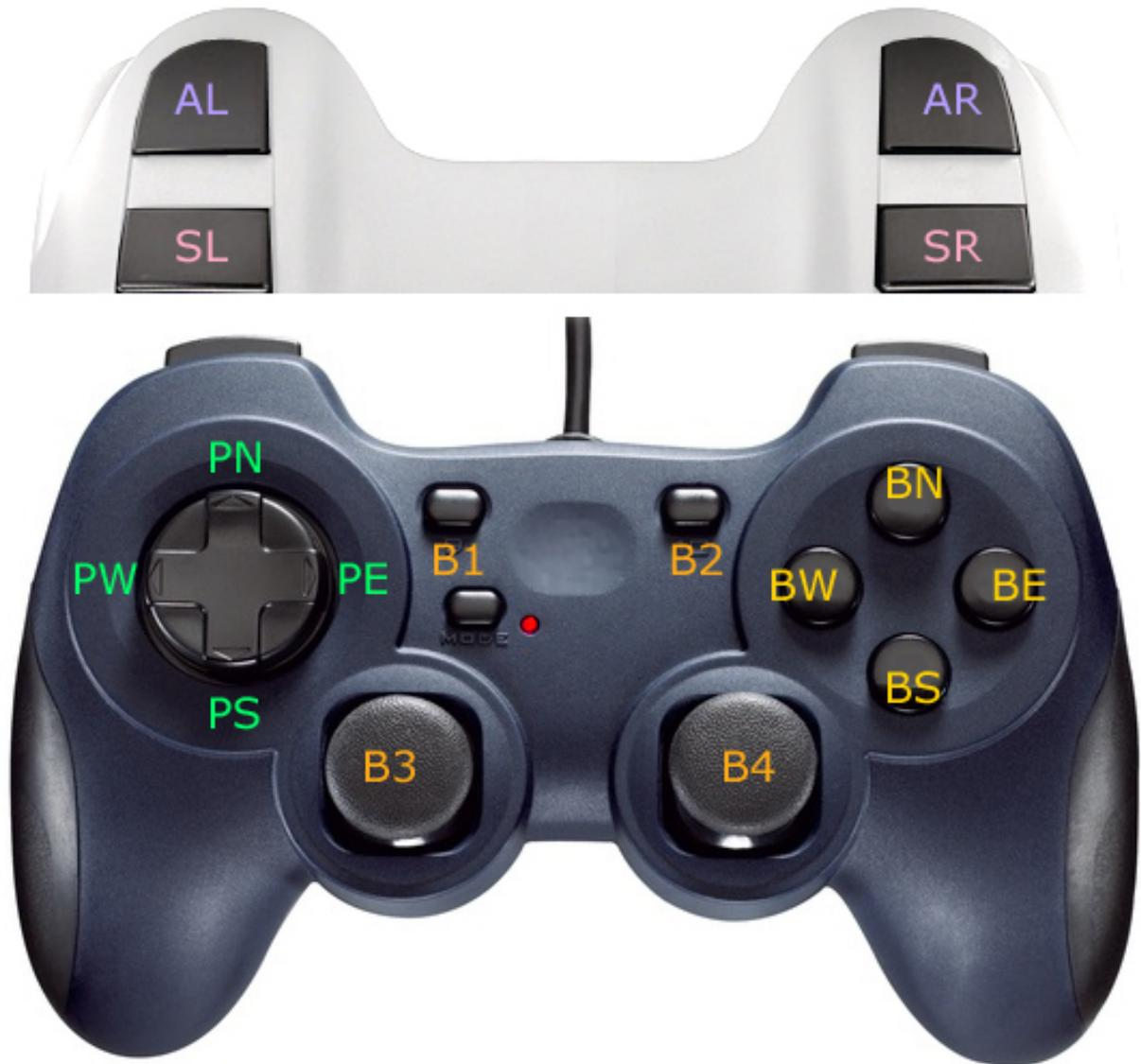
The JoyPad plugin supports up to 16 buttons, including SL, AL, SR and AR buttons (an ordinary gamepad has 12 buttons, including the POV and excluding the front buttons). All of which can be programmed alone or in combination with the "Safe" and/or "Alt" buttons, to any build in function supported by Mach3 (See Appendix F).
